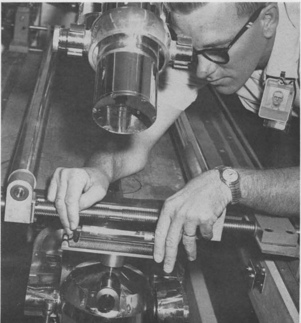
ADJUSTING the radiation source holder on the DXT Machine is Harry Olson (8115-1). DXT means
